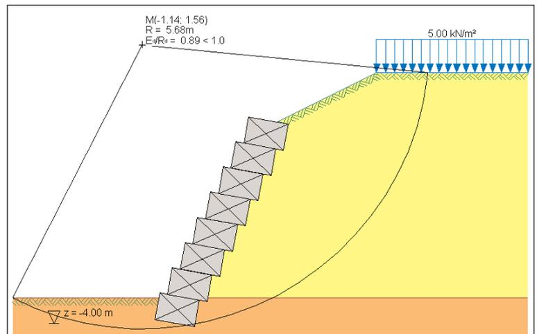
Inclined layered blocks with offsets
