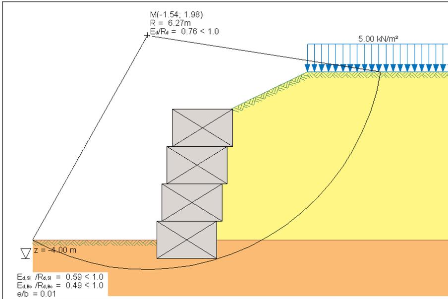
Display of the foundation engineering checks
