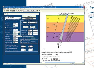
Input of the pile parameters and verification
