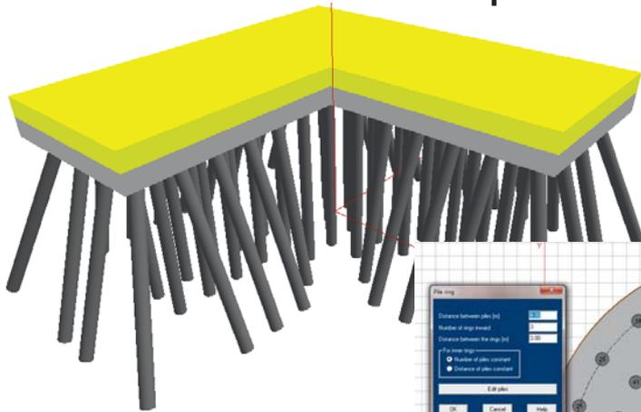
Foundation raft with pile grid incl. inclined piles, 3D preview of the system
